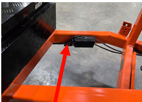
4-Pin connector for wireless transmitter (Front of machine on inside of hitch)
