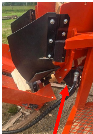
4-Pin connector for wired lights (Rear of machine under auxiliary hydraulic ports)
