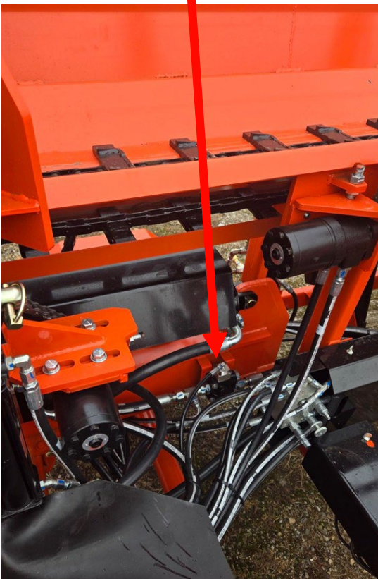
MSL Valve Location
